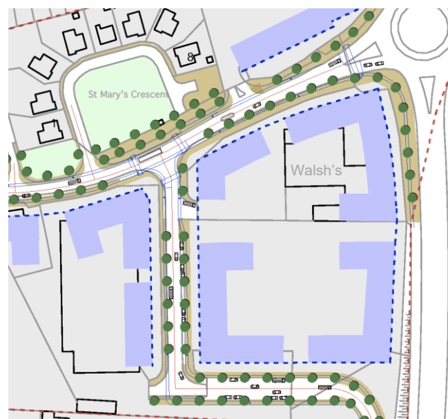
Ring road junction and extension of access road for the industrial estate
