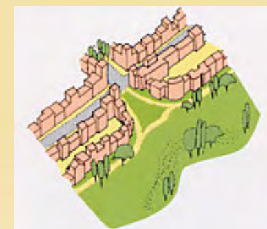
Fig. 3.07 Public spaces should have development fronting onto it, to define the space and promote passive supervision.
