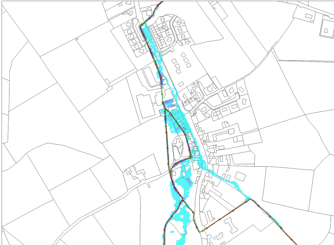
Fig 11.6 Extent of flooding through settlement of Ballyhale. Extract from Hydraulics Report prepared by McCloy Consulting Engineers.
